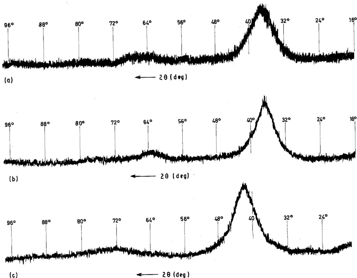
Figure 2 Diffractometer pictures of amorphous splats in (a)  $Zr_{72}Pd_{23}B_5$ , (b)  $Zr_{75}Pd_{20}Si_5$  and (c)  $Zr_6Ru_{60}Si_{28}$  ternary systems.
