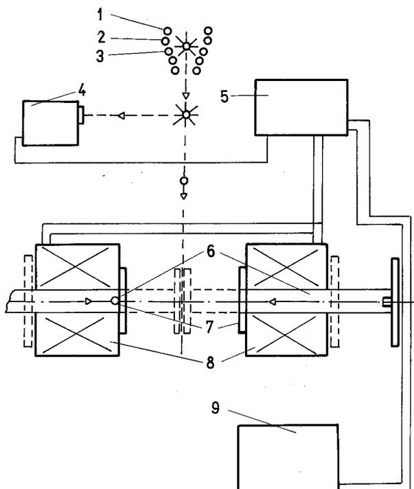
Figure 1 Schematic drawing of the splat-cooling technique. 1, r.f. stabilization ring; 2, r.f. coil; 3, levitating sample; 4, detector; 5, control unit; 6, high-velocity two-piston arrangement; 7, copper-pistons; 8, solenoids; 9, power supply.
